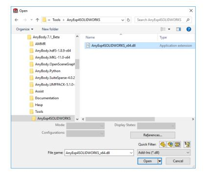
The AnyExp4SOLIDWORKS DLL can be found in the AnyBody installation, ypically in the folder [C:Program FilesAnyBody TechnologyAnyBody.X.XToolsAnyExp4SOLIDWORKS], where X.X indicates the AnyBody version number.
