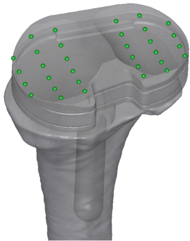
Reaction elements on the surface of tibial insert
