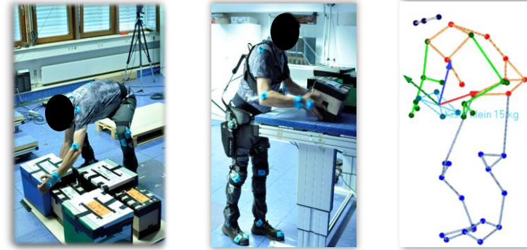
Test person during the laboratory study and marker model from motion capture (Qualisys)
